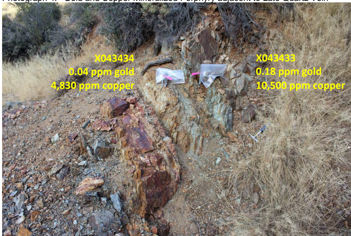
Photograph 4. Gold and Copper Mineralized Porphyry adjacent to Late Quartz Vein
