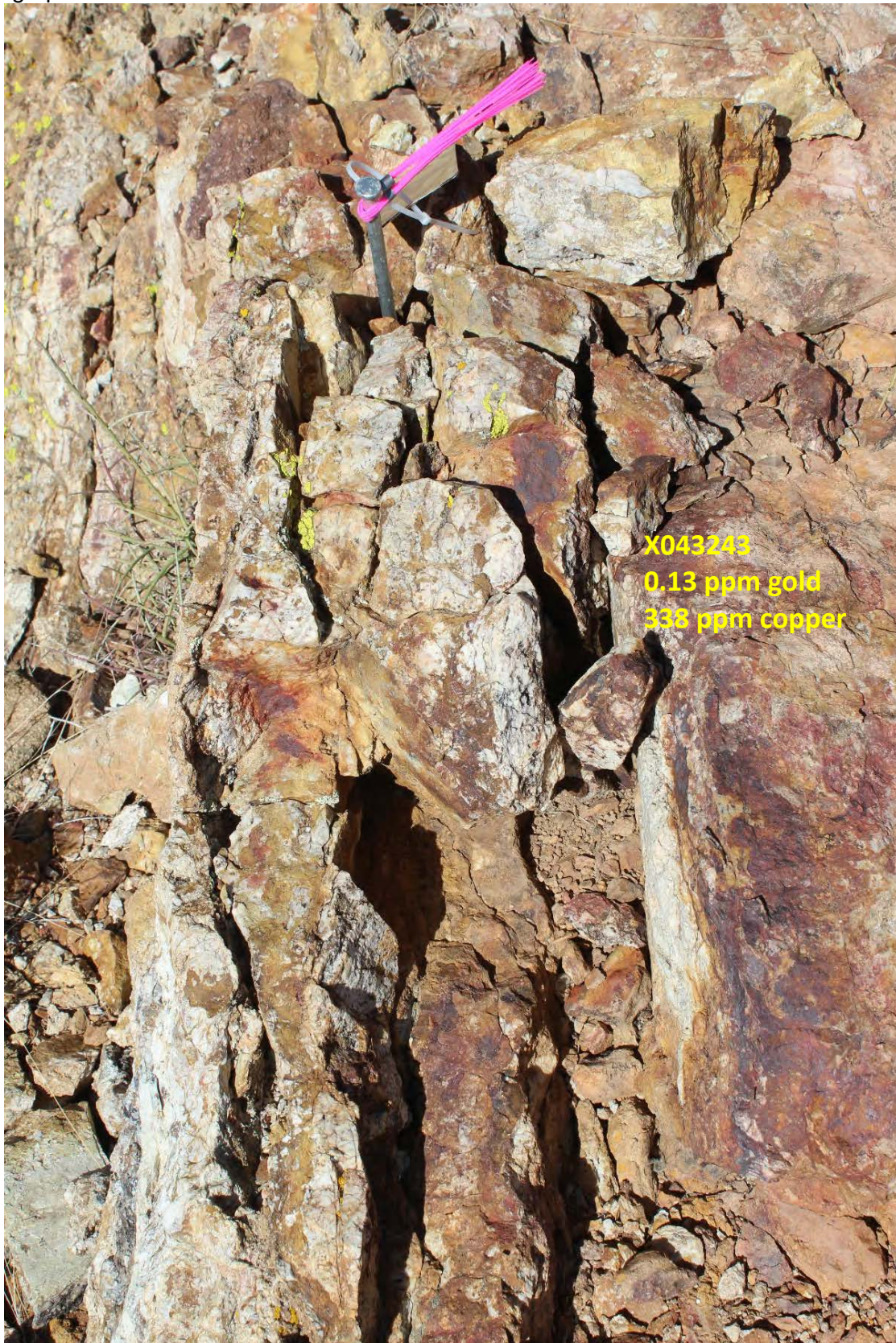
Photograph 11. Laminar Quartz Veins – Jewell Tunnel Air Vent
