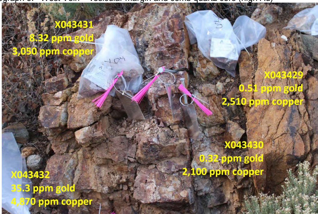
Photograph 9. West Vein – vesicular margin and comb quartz core (high Au)
